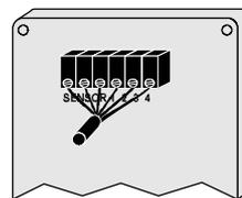
**Note:** All external cables connector to the rear panel should be ended with cable lugs.
