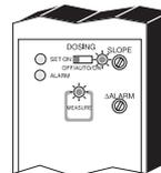
If the dosing switch is in ON position the DOSING relay is always activated and the SET ON LED lights up; the ALARM relay is activated and the ALARM LED blinks according with the input reading, setpoint and ALARM threshold.
