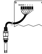
The DIN connector has to be removed when this probe is used in conjunction with an **HI 8936** transmitter. See page 21 for the proper connection scheme.
