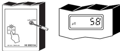
Use a small screwdriver to adjust the "ΔALARM" trimmer until the desired tolerance is displayed.
