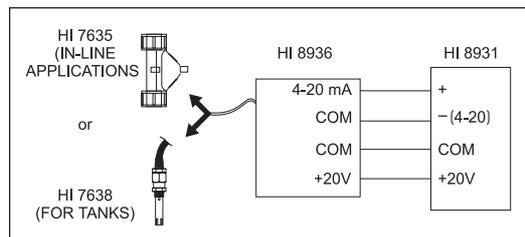
Use a PVC insulated 4-core cable to connect the transmitter to the HI 8931 conductivity controller (see also page 22).
