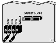
The regulated DC supply required for the proper functioning of the circuit is marked "+20 V" and "COM", and the transmitter current output is indicated "4-20 mA" and "COM".
