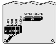
The regulated D.C. supply required for the proper operation of the transmitter is "+20 V", labeled "+20 V" and "COM". The current (mA) output terminals are labeled "4-20 mA" and "COM".
