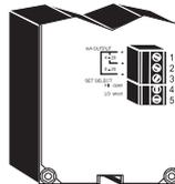
Connect the “+” wire from the recorder to terminal 1 on the instrument and the other wire (common) to terminal 2 for 4-20 mA recorder output or terminal 3 for 0-20 mA recorder output.
