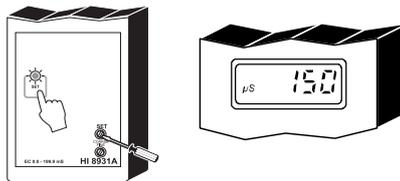
Use a small screwdriver to adjust the COARSE and FINE trimmers until the desired value is displayed.
