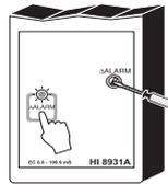
When an alarm occurs, the "ALARM" LED lights up.
