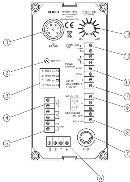
1. DIN connector for EC probe
