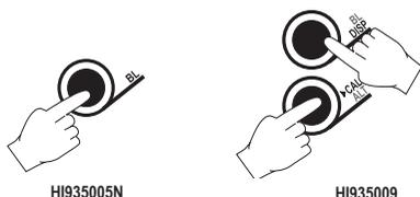
**Note:** The backlight automatically shuts off after approximately 1 minute with no buttons pressed.
