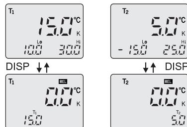
In relative mode, the main body of the LCD shows the difference from the reference temperature. The lower portion displays the current temperature for the selected channel.
