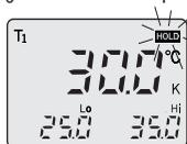
**Note:** Although the display is frozen, internally the meter continues measuring and updating Hi/Lo and relative values.
