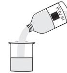
Use the 1413  $\mu\text{S}/\text{cm}$  solution at HI 983303, 1382 ppm for HI 983306, 5.00 mS/cm for HI 983307, 6.44 ppt for HI 983308 or 800 ppm for HI983309.
