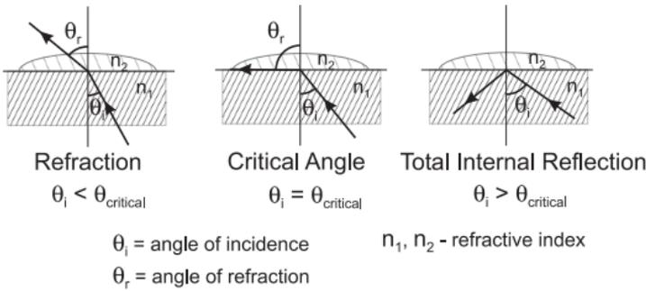
In the [HI96812](#), light from an LED passes through a prism in contact with the sample. An image sensor determines the critical angle at which the light is no longer refracted through the sample.
