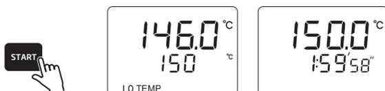
The end of the digestion time is signalled by an acoustic signal (5 short beeps) and "DONE" message is displayed. The heating is turned off and the block begins to cool off.
