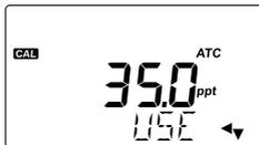
4. Used standard is automatically recognized. When the standard is recognized “REC” is displayed. “WAIT” is displayed until the reading is stable and the calibration is accepted.
