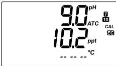
Temperature sensor not reading correctly.
