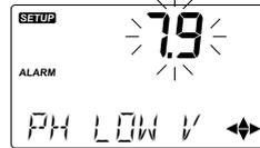
With Low Alarm configured as enabled "PH LOW VALUE" is scrolled on the bottom of the LCD. Actual pH value (editable) is displayed blinking.
