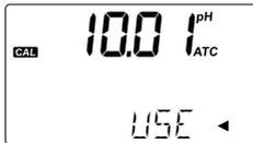
6. Place the electrodes in second calibration buffer.
