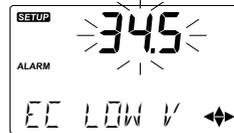
With EC Low Alarm configured as enabled "EC LOW VALUE" is scrolled on the bottom of the LCD. Actual EC value for low alarm (editable) is displayed blinking.
