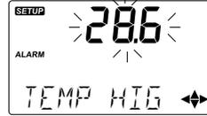
With Temperature High Alarm configured as enabled "TEMP HIGH VALUE" is scrolled on the LCD. Actual high alarm temperature value (editable) is displayed blinking.
