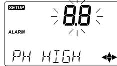
With pH High Alarm configured as enabled "PH HIGH VALUE" is scrolled on the bottom of the LCD. Actual pH value (editable) is displayed blinking.
