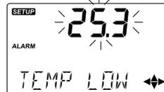
With Temperature Low Alarm configured as enabled "TEMP LOW VALUE" is scrolled on the LCD. Actual low alarm temperature value (editable) is displayed blinking.
