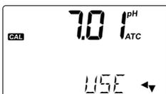
3. Place the electrodes in 7.01 pH or 10.01 pH buffer solution.
