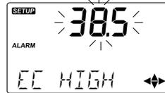
With EC High Alarm configured as enabled "EC HIGH VALUE" is scrolled on the bottom of the LCD. Actual EC value for high alarm (editable) is displayed blinking.
