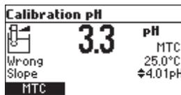
The evaluated slope is more than the highest accepted value (110 % of default slope).
