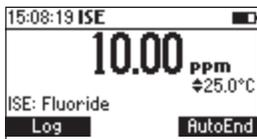
The "ATC" (or "MTC") message is turned off because ppm readings are not temperature compensated.
