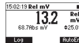
**Note:** If using the pH electrode while in mV mode, the instrument will measure the mV generated by the pH electrode.
