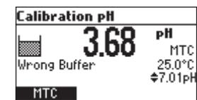
The pH reading is not within range of the selected buffer. Select another buffer using the **ARROW** keys or change the buffer.
