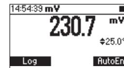
The "ATC" (or "MTC") message is turned off because mV readings are not temperature compensated.
