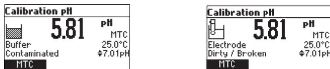
The offset of the electrode is not in the accepted range. Check if the electrode is broken or clean it following the Cleaning Procedure (see page 58). Check the quality of the buffer. If necessary, change the buffer.
