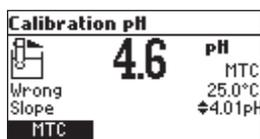
The evaluated slope is less than the lowest accepted value (80% of default slope).
