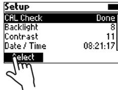
3. Follow the prompts on the screen. The meter will prompt to measure each cuvette provided in the Hanna Instruments® CAL Check Standards kit. To exit the process at any time, press **ESC** key.
