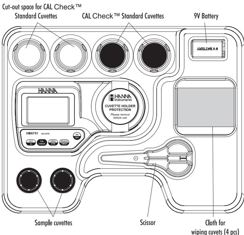
The **HI96751** is an auto diagnostic portable microprocessor meter that benefits from Hanna Instruments' years of experience as a manufacturer of analytical instruments. It has an advanced optical system based on a Light Emitting Diode (LED) and a narrow band interference filter that allows most accurate and repeatable readings. All instruments are factory calibrated and the electronic and optical design minimizes the need of frequent calibration.
